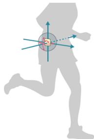
The device is equipped a GPS and 9-axis sensor that measures every step of the run, including distance, pace, pitch, stride and other general running metrics. It also provides more than 20 metrics on form
