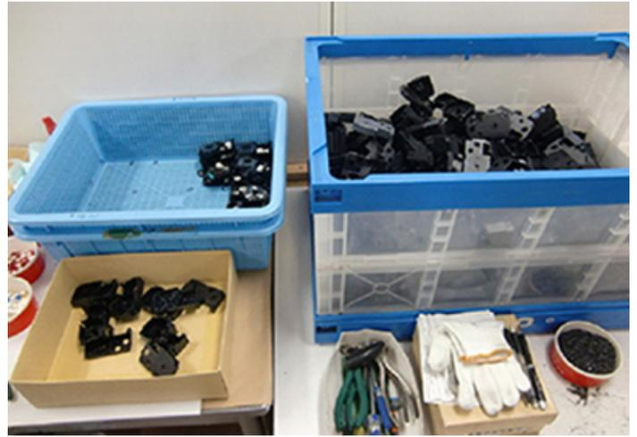
Disassembly and separation of tape cartridges and ink ribbon cassettes
